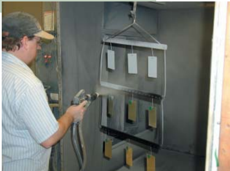
Worker spraying powder coat on test panels.
